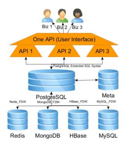
Fig. 1. Framework of the unified access layer system
